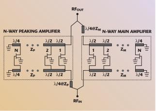
Fig. 2 Schematic of a new N-way distributed Doherty amplifier.
