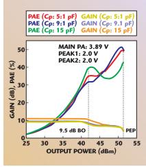
ightharpoonup Fig. 9 Measured PAE and gain as a function of the shunt capacitance  $C_M$ .
