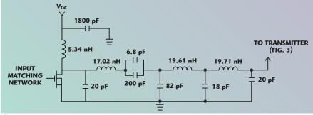
▲ Fig. 2 Practical broadband class E parallel circuit combined with a reactance compensation technique.
