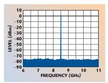
▲ Fig. 7 Measured output spectrum of the prototype self-offset PLL.
