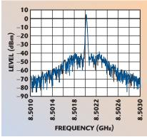
▲ Fig. 6 Measured close-in spectrum of the prototype self-offset PLL.
