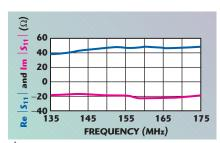
▲ Fig. 5 Measured input impedance of the elliptical harmonic filter with the series Lx Cx network.
