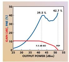
Fig. 8 Measured PAE and gain performance of the proposed three-way distributed Doherty amplifier.
