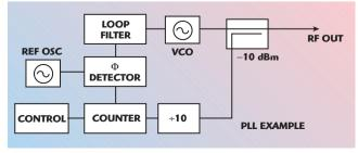
Harmon- ▲ Fig. 7 Block diagram showing an example of a PLL.
