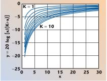
▲ Fig. 3 Phase noise improvement due to reduction in the main divider's division ratio.
