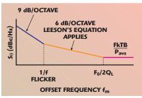
▲ Fig. 3 Phase noise plot showing determining factors.<sup>6</sup>
