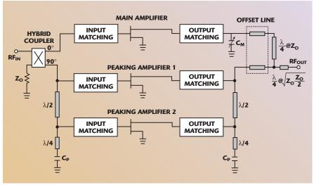
Fig. 5 Schematic of the proposed three-way distributed Doherty amplifier.
