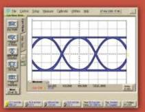
WAVEFADE" filter yields symmetrical eye diagram with minimal ringing and group delay distortion.
