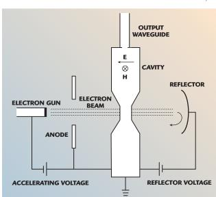
▲ Fig. 2 In a reflex klystron, the beam is first velocity-modulated in a microwave cavity, then reflected back into the cavity to provide feedback necessary for oscillation. As the cavity is part of the body of the tube, it is necessarily at ground potential and a negative voltage is applied to the cathode.
