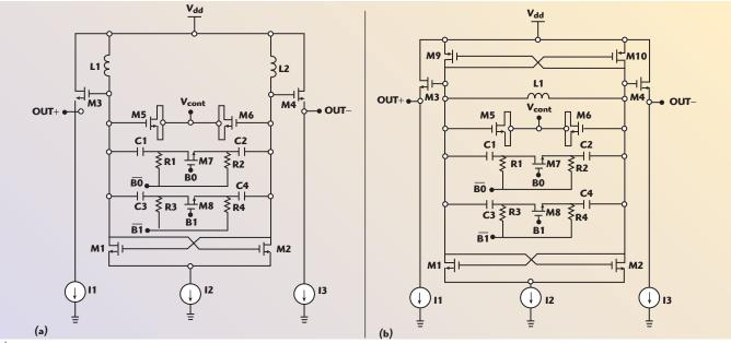
Fig. 5 VCOs; (a) NMOS only and (b) complementary CMOS.
