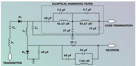
▲ Fig. 3 Schematic of the series LC network with an elliptical harmonic filter and RF switching of the 135 to 175 MHz range.
