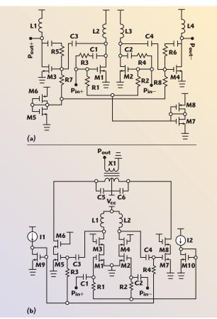
Fig. 2 CMOS PA; (a) differential and (b) cascode differential.
