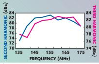
Fig. 7 Measured second- and thirdharmonic levels across the frequency band.
