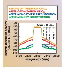
▲ Fig. 11 Measured WCDMA one-carrier spectrum of the three-way Doherty amplifier.
