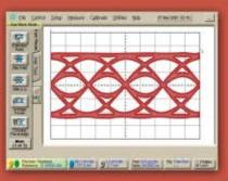
40 Gb/s duobinary signal created using a 12 GHz WAVEFADE" filter.
