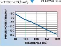
Fig. 1 Typical phase noise
