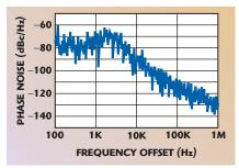
Fig. 1 Phase noise of a 6.7 GHz phase-locked oscillator.
