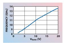
Fig. 5 Tuning characteristics with a tuning voltage of 0 to 20 V.
