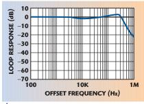
Fig. 8 Measured closed-loop response of the prototype self-offset PLL.
