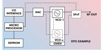
▲ Fig. 6 Block diagram showing an example of a DTO.
