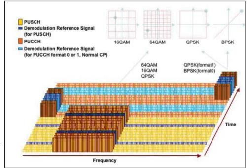
**Figure 7** Frame Structure 1 for the uplink showing one subframe vs. frequency
