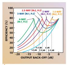
▲ Fig. 4 Calculated efficiency of the N-way Doherty amplifier at various back-off powers.
