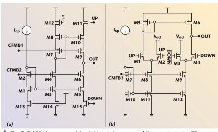
▲ Fig. 7 CMOS charge pump; (a) switching at the source and (b) current steering CP.
