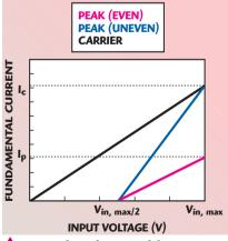
▲ Fig. 3 The Doherty amplifier's fundamental current vs. input voltage.
