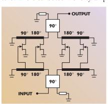
Fig. 1 Diagram of a conventional balanced dual-fed distributed amplifier.
