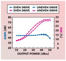
Fig. 8 Gain and power-added efficiency vs. output power.
