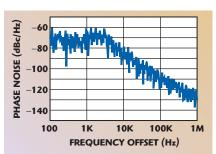
▲ Fig. 2 Phase noise of a 13 GHz phaselocked oscillator.
