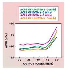
▲ Fig. 9 ACLR performance for two-tone signals spaced ±5 MHz.
