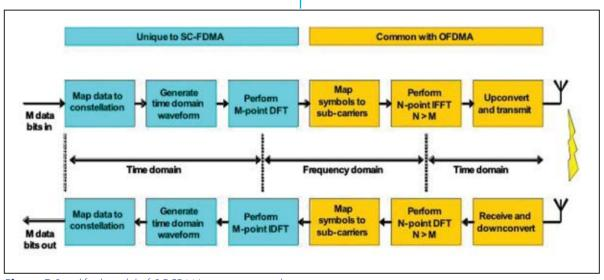
Figure 5 Simplified model of SC-FDMA generation and reception
