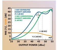
Fig. 6 Simulated PAE and gain performance of the proposed three-way distributed Doherty amplifier.
