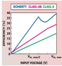
Fig. 2 Efficiencies of the Doherty, class-A and class-AB amplifiers.
