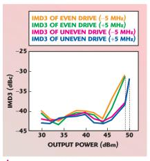
Fig. 10 IMD3 for two-tone signal with ±5 MHz spacing.
