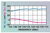
▲ Fig. 4 Measured real and imaginary input impedance of the elliptical harmonic filter without the series Lx Cx network.
