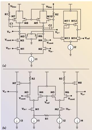
Fig. 4 AGC; (a) variable transconductance and (b) variable biasing.
