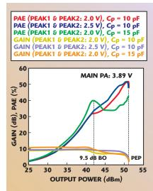
Fig. 10 Measured PAE and gain variation as a function of Cp and peaking amplifier's bias.
