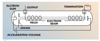
▲ Fig. 3 A backward-wave oscillator is similar in many respects to a travelling-wave tube, but it makes use of a backward wave that propagates on the helical slow-wave structure. This provides feedback necessary for oscillation.
