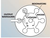
▲ Fig. 1 A magnetron is one of the simplest and earliest microwave tubes. Electrons emitted from the cathode are accelerated toward the anode, but a magnetic field causes them to spiral in the space between those elements. The spiraling electron cloud excites fields in the coupled cylindrical cavities in the anode.
